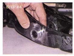
ing surface. Do not apply grease before any welding.
