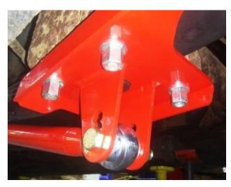
23. Adjusting the length of the traction bar tube must be completed when the vehicle is on the ground and sitting at ride height.
