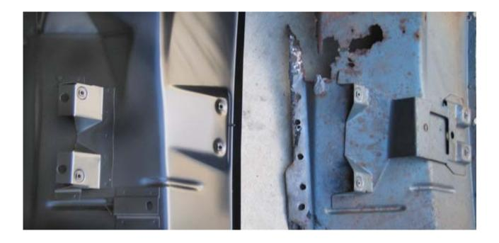
After taking some measurements, the upper mounting holes on the new piece are flanged such that the height is the same as the bracket on the 65 piece. Using the 67/68 brackets, the wiper motor bracket mounts in the same plane as on the 65. The only issue is that the lower mounting hole pattern is about 1/2" narrower on the 67/68 than on the 65. I drilled two new holes in the motor bracket and slotted the area to allow for some adjustment. Wiper motor and arms mounted fine with no binding.
