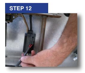
Insert the wire connector into the motor. You should hear the locking tab snap into place.
