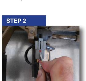
Carefully push down and out on the red plastic locking block.
