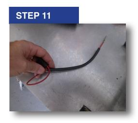
Insert both wires back into the black protective sleeve.
