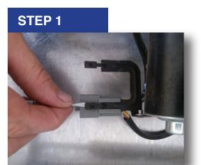
Remove the gray electrical connector from the pronged bracket. Gently lift up the metal tab and pull the connector off.
