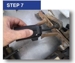
Mount the new motor with the electrical socket downward. If you put the socket on top, your seat will bottom out on it and damage the plastic.
