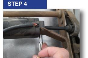
Remove the ¼" head screws holding the motor to the frame.
