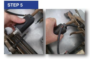
Pull the motor away from the frame to disengage the flexible drive shafts.
