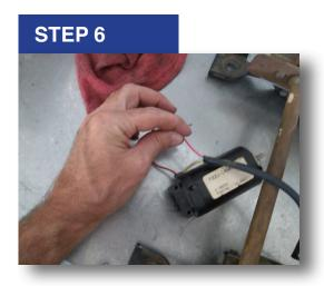
Pull the electrical wires out of the black protective sleeve.
