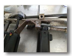
Use a long screwdriver or pry bar, push downward to help compress the gas cylinder. Align the mounting holes and insert a 1/4" bolt or similar object to hold the new motor in the correct mounting position.
