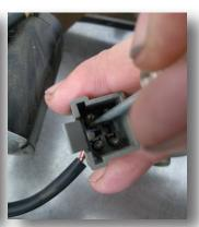
Gently lift the locking prongs and pull the connectors out the back of the connector as shown.
