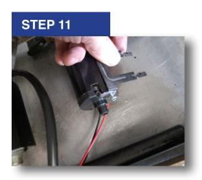
Drill out or grind off the rivet holding the three pronged bracket to the old motor. Install the pronged bracket onto the new motor as shown and secure with the supplied screw. Slide the grey connector back onto the prong.
