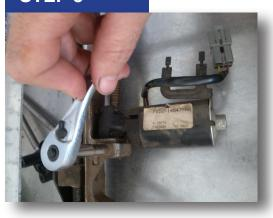
Remove the ¼" head bolt and lift off the L-shaped bracket.
