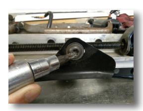
Remove the T45 torx head bolt holding the forward/backward slide bracket to the threaded block. Lift the threaded shaft up to get clearance to the roll pin end protruding into the forward/backward shaft channel.
