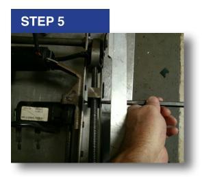
Use a long punch and drive the roll pin out. Once the roll pin is out, the seat frame will fully extend in the up position.
