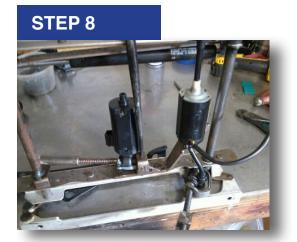
Use a hammer and long punch to drive the roll pin back into the seat frame. Let the roll pin push out whatever holding mechanism you used in step 7. Do not hit the roll pin directly with the hammer. Trying to hammer the roll pin directly will result in accidental strikes to the motor housing and possibly damaging it.
