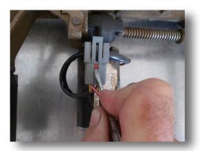
Lift up the metal tab to disengage the locking mechanism. Then push out the red lock block from the gray connector.
