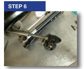
Unscrew the old motor and shaft assembly from the tube nut. Screw the new motor back into the tube nut about the same number of turns needed to remove it. Twelve full turns in will work.
