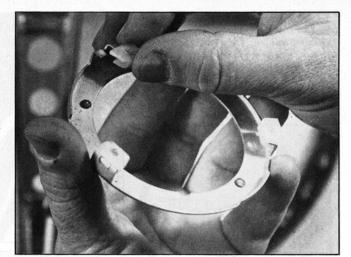
Next, slip on plastic "feet" for outer ring contact.
