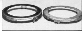
Here is the reason we needed shims—and your wheel very well may too. Notice ring on the left—from an original wood wheel—which is taller than one on the right which was sent to us. That's why shorter contact rings needs to be shimmed.
