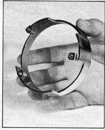
This chromed plastic spacer ring fills gap between end of steering column and base of horn button assembly.
