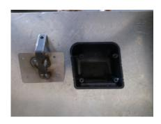
2. Attach the supplied switch harness to the power switch as shown.
