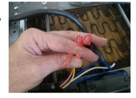
7. Attach the three prong connectors together. The cut off ends will need to be spliced into your car. The two wires that are the same color(one has a strip) are the grounds. The odd wire(white) is the power. Hook the power to a fused 12v power source.
