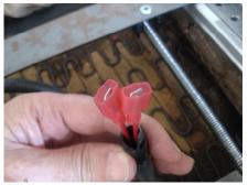
6. Plug the motor leads into the female ends of the supplied harness. The wire
