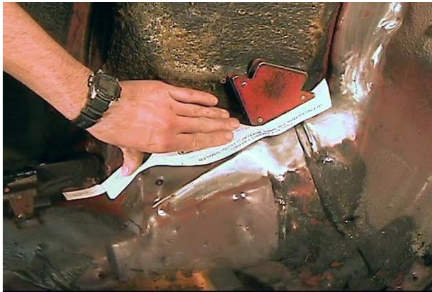
Figure 4 – Inner Wheelwell Front Template
