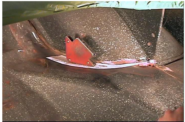
Figure 5 – Inner Wheelwell Rear Template
