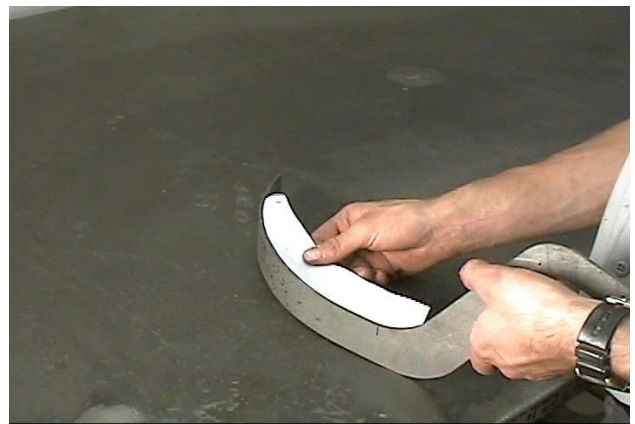
Figure 12 - Rear Template Bend Profile
