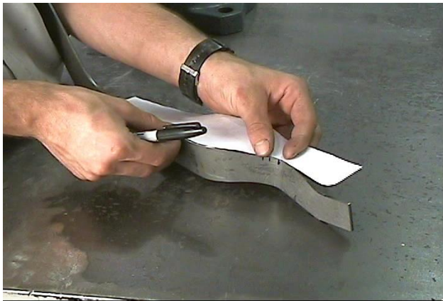
Figure 11 - Front Template Bend Profile
