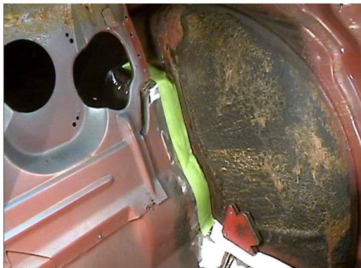
Figure 6 – Cut Line Extension Using 2" Tape
