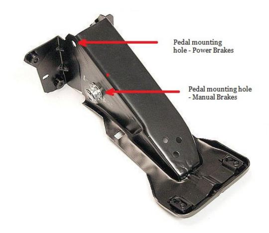
The Ford factory brake pedal support contains two mounting positions for both the original manual brake pedal and the power brake pedal. The new power brake pedal will mount in the upper hole located closest to the firewall. This position ensures proper leverage to actuate your brake system with comfortable pedal pressure.
