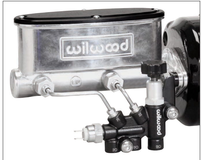
Photo 1. Proportioning Valve Bracket Kit Final Installation (left hand shown)
