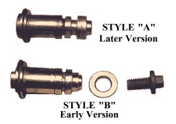
You must determine which style of valve you have in order to get the correct seal kit. You must then compare the seals in the kit and the old seals to make sure they are of the correct diameters for your valve.
