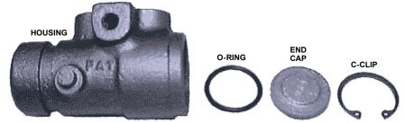
STEP 3: Remove C-Clip, End Cap and O-Ring.
