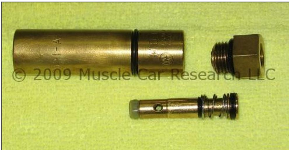
Lubricate the seals with brake fluid and insert the proportioning valve piston (the brass piston in the picture) into the valve body as far as it will go. *If everything is installed properly you should*
