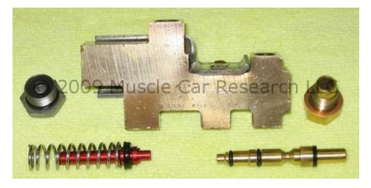
Install the spring behind the proportioning valve piston. Place the metal spring cap on top of the spring (the ridges on the cap fit *inside* the spring) and install the steel plug. Tighten the plug only enough to form a positive seal with the o-ring. Install the warning lamp switch.
