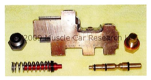
Install the spring behind the proportioning valve piston. Place the metal spring cap on top of the spring (the ridges on the cap fit *inside* the spring) and install the steel plug. Tighten the plug only enough to form a positive seal with the o-ring. Install the warning lamp switch.
