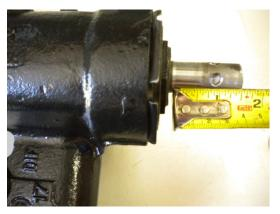
4. Using supplied U joint (1"DD x ¾" smooth), drill 3 holes (drill bit provided) at 90 degrees and 7/16"deep tap with a supplied tap, install set screws with thread lock provided. (Can also be welded).
