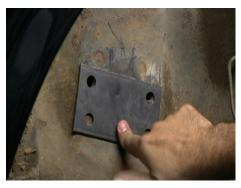
Be sure that you have ordered the correct kit! The 1965-66 plate is shown above. Note the slight offset of the holes. The 1967-73 plates will have the holes set directly over each other.
