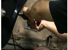
Mark the center of the hole with a centering punch if available. Then drill a pilot hole using a 1/8-inch drill bit.
