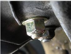
Use a washer between the original shock tower control arm bolt and the inner shock tower's new hole. Reuse the original shims. Due to the new plate and position you will probably need less shims. On all applications these nuts will need to be tightened to 80-100 ft- lbs.
