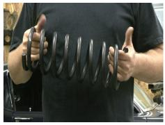
National Parts Depot recommends installation of a GT or higher spring rate in order to maximize the performance kit.
