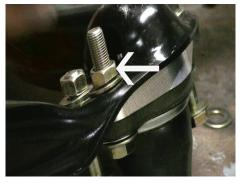
Bolts install from the bottom and the angled nuts are installed as shown. Rear bolt in photo is installed to position the angle plate. It is important that the angled nuts angled bottom surface remain flat to the washer and control arm surface during all tightening. Hold the nut (arrow) in place with a wrench then tighten the bolt. The bolt is final tightened to 38-42 ft-lbs.
