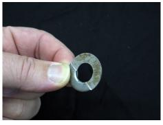
The shock tower on 1967-73 Mustangs will have multiple layers of metal to pass through, use the step washers shown to achieve correct fitment.
