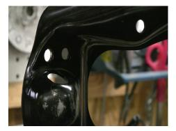
Drill the bolt holes on the upper control arm out to 3/8 or 13/32-inch.
