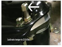
Locking nut (arrow) tightens to 25 ft-lbs. after all four (or in the case of a 3-bolt control arm, three) mounting bolts are torqued.
