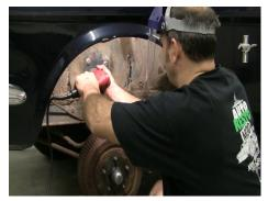
For the final drilling use a ½-inch cobalt bit.
