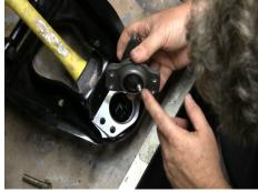
The plate sits as shown ('65-'66 installation shown, 1967-73 typical). Make sure that the new ball joint that comes with the kit is installed with the zerk fitting facing the opening in the ball joint cap.
