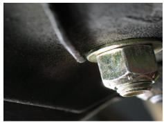
On some 1965-'66 Mustangs there may be interference between the lip of the stiffening plate in the engine bay and the washer. Clearance the stiffening plate so the washer will sit flat.
