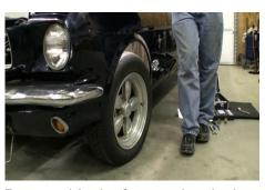
Reassemble the front end and take the car to a qualified alignment shop. It is recommended that you trailer the car or only drive for very short distances (five miles or less) in order to prevent excessive tread wear.
