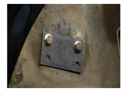
The plate sits flush to the shock tower as shown. On the '65-'66 plate the new holes are toward the
