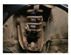
Be sure to safely remove the front suspension using a coil spring compressor that is approved for this type of coil. Do not use a McPherson strut coil spring compressor for this job. Take appropriate precautions when removing the spring.
