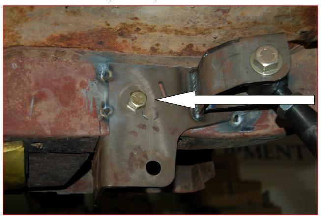
3. Tack the forward frame brackets into place as shown in the picture above and remove the bolt.
