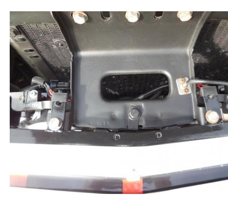
I had to "clearance/grind" some of the bottom material off of the support to make it fit, but that's no big at all (although I clearanced both sides, here's a shot of the support with one side clearanced, for reference).
