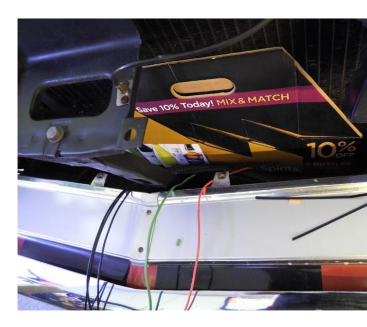
The install is very straight-forward. THE MTF grill sits on top of your grille molding, instead of behind it like the OEM grille. The new MTF grille fits perfectly, with virtually no "gaps" anywhere – a sure sign of excellent build quality. There are six attaching points available to use, but I only used/needed two of them, located on the top/middle of the grille, to attach to the hood latch support. The grille itself is pretty stout, so I didn't feel the need to use all of the attaching points.
