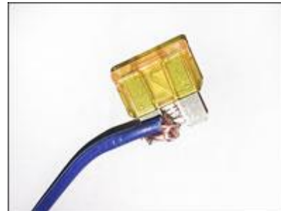
Wire Jammed Into a Fuse
