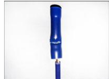
Broken Butt Connectors
