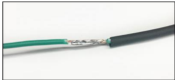
Soldered Connection w/ adhesive heat shrink
