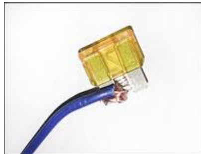
Wire Jammed Into a Fuse
