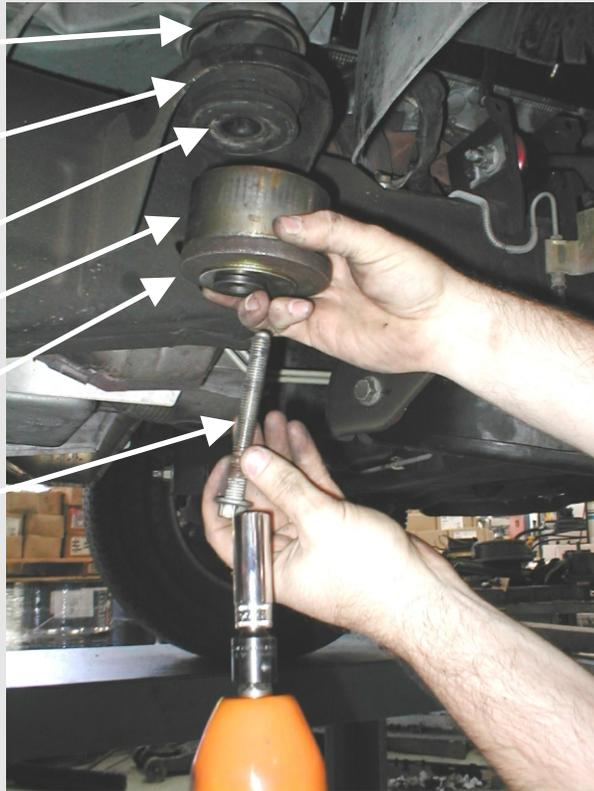
**NOTE:** Be sure on disassembly to note the quantity and positions of any shims that may have been inserted for body alignment. These shims will have to be reused to insure proper body alignment.
