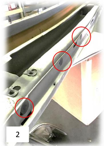
Figure 2: Factory rear bumper push pins
