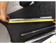
VI. Cut the shaft on the slip joint side, measuring up 18".
