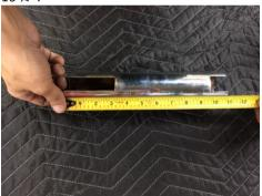
V. Cut the column on the steering box side, up at 22 5/8".
