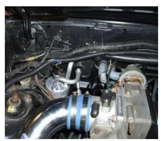
19. The suction hose is pre-crimped on the accumulator and will be routed as shown to the large suction fitting on the compressor. Install and lubricate the correct size o-ring and attach to the compressor.
