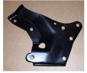
7. Replace the front mounting bracket on the engine using the original hardware. Using the supplied hardware, install the adapter brackets on the factory brackets as shown. Bolt the front adapter behind the front factory bracket, and the rear adapter (they are identical) to the front of the rear factory bracket. Do not tighten these bolts yet.
