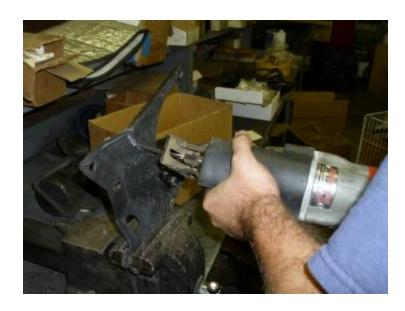
The photo at left shows the piece trimmed from the original mounting bracket.
