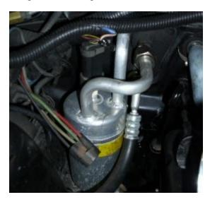
The discharge hose connects the compressor to the condenser. Install & lubricate a correct size o-ring to the 45' fitting and install on the compressor discharge fitting. Make certain you orient the fitting at the compressor end as shown to clear the distributor. Tighten the fitting upon positioning.
