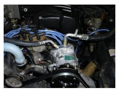
13. Install & lubricate the correct size oring on the suction hose and attach to the suction fitting on the compressor.
