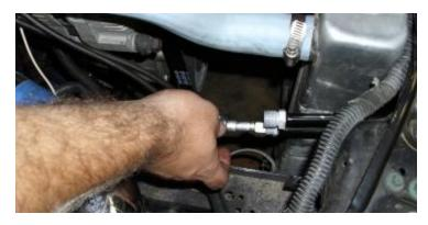
22. Install & lubricate the correct size oring on the straight end and connect the straight fitting to the condenser at the core support. Do not tighten fittings yet.
