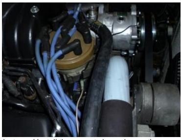
24. Lubricate and install the correct size o-ring on the straight fitting and connect to the top fitting of the condenser. Tighten the fitting.
