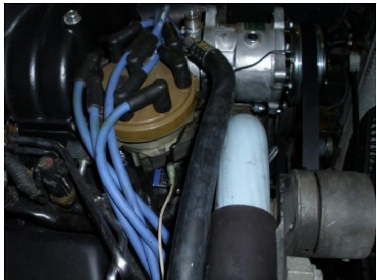
Install & lubricate the correct size o-ring on the suction hose and attach to the suction fitting on the compressor.
