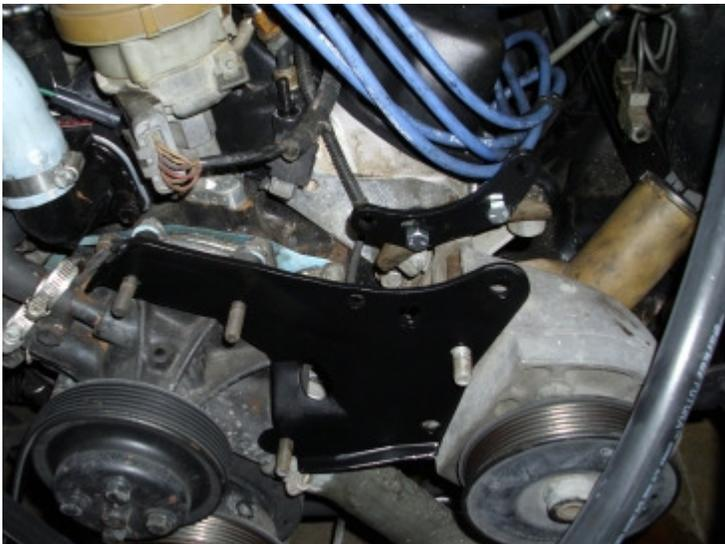
12. Replace the front mounting bracket on the engine using the original hardware. Using the supplied hardware, install the adapter brackets on the factory brackets as shown. Bolt the front adapter behind the front factory bracket, and the rear adapter (they are identical) to the front of the rear factory bracket. Do not tighten these bolts yet.
