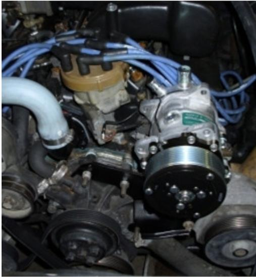
13. Using the supplied hardware, install the compressor as shown. Attach the clutch wire.
