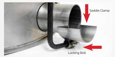
Use the hanger and saddle clamp for the outlet of the muffler. Slide the hanger through the corresponding rubber grommet on the chassis then snug the hanger into the saddle clamp and tighten the locking bolt to hold the hanger in place.
