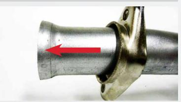
Slide the flared flanges over the head pipes so that the flared end of the flanges match the flared end of the head pipes as shown.
