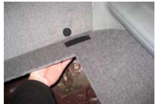
1. The two storage compartment lids fit over the lower bins as shown in the photo. The Velcro strips align to hold it in place. You're Done
