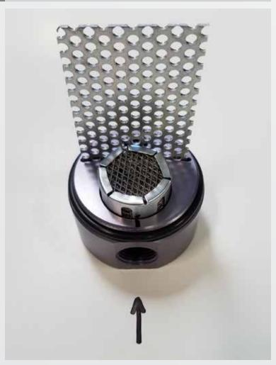
When assembling the oil separator place the 11 ¾ long hose on the draw-side of oil separator as shown in picture. This hose will mount to the intake side of engine.
