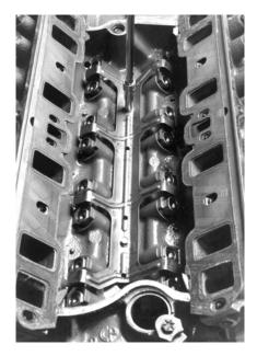
The installation of your COMP Cams® Ford 302 HO Hydraulic Roller Lifter Kit is now complete. Refer to the camshaft installation and degreeing instructions that came with your cam for further instructions on pushrod installation and valve adjustment that are needed to complete your project. Order COMP Cams® Camshaft Degree Kit (Part #4796) to make these adjustments easier.
