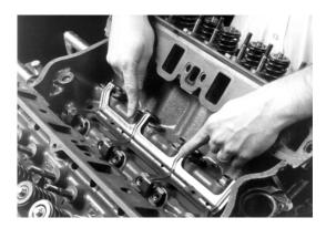
pairs and riding on the raised ball area of the lifter guides before marking the hole locations. Mark the holes with a center punch, remove the retainer, and drill and tap the holes as necessary. Do not allow any metal shavings created during the drilling and tapping process to remain in the engine. Severe engine damage may result.
