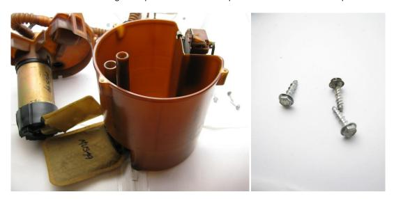
2 – remove the OE sock and isolator from the OE pump and install on the DW65c
