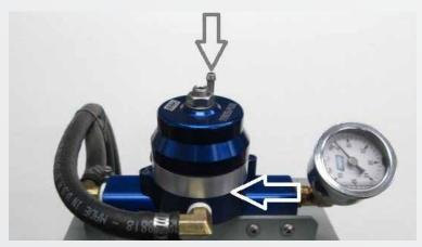
Now that the fuel system has been pressurized it is a good time to check for leaks around the BBK Fuel Regulator
