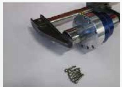
With the Fuel Regulator clamped firmly it releases then tension on the screws remove the six screws on the bottom of the Fuel Regulator.
