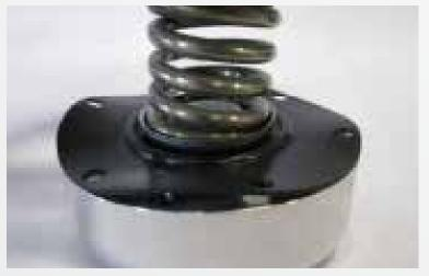
Take the new spring that is supplied in the kit and place it onto the spring locating cup on the diaphragm.
