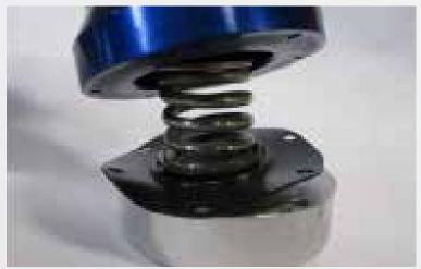
Place the spring cap on top of the spring with the pointed side facing down. With all the components together place the top portion of the Fuel Regulator on top. NOTE: While firmly holding the two half's together. Start the six screws into the bottom of the Fuel Regulator.
