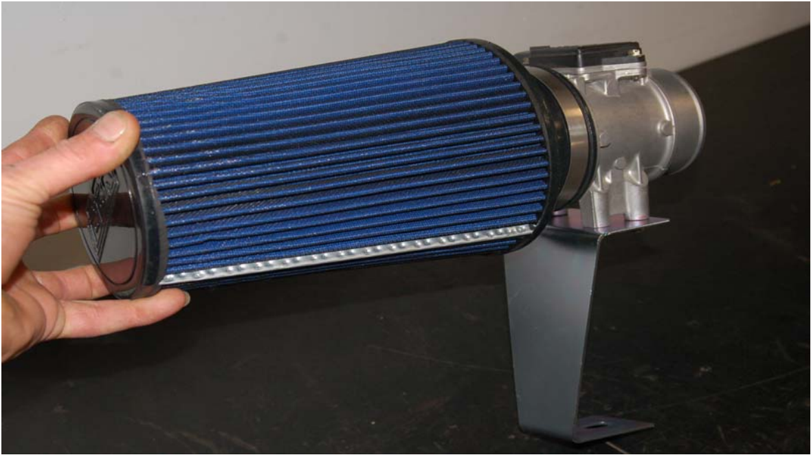
Fig. 5 BBK Kit # 1556 bracket shown installed on Mass Air housing. Air Filter also shown installed.
