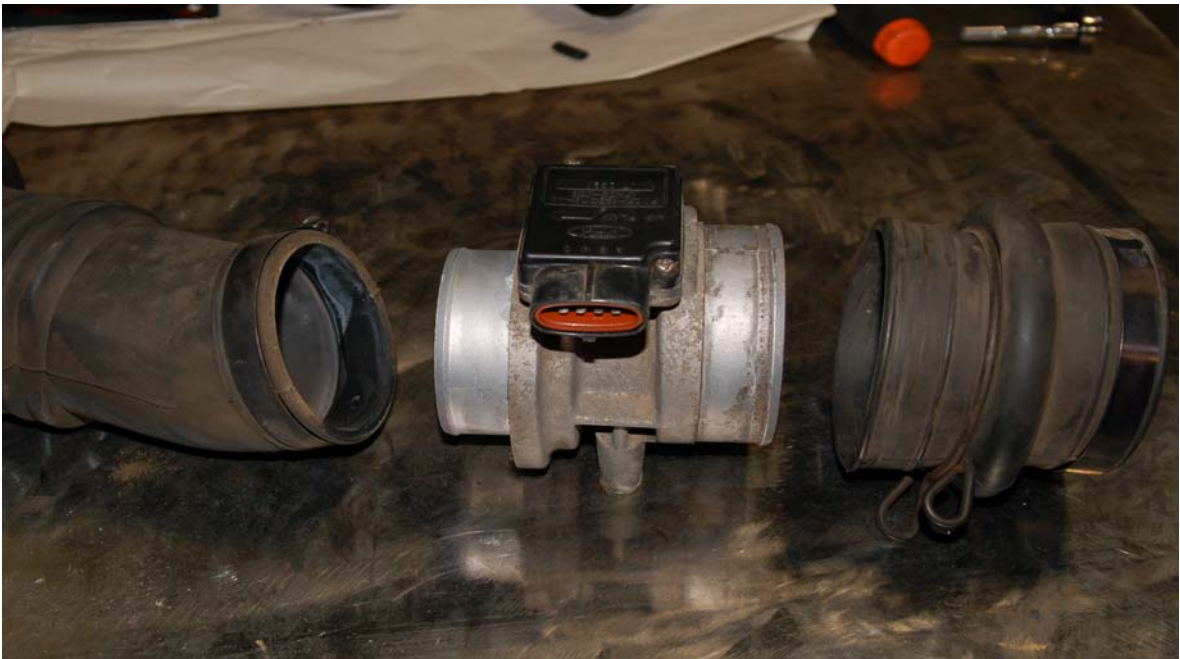
Fig. 4 Remove Mass Air Sensor housing from the stock inlet tubes.
