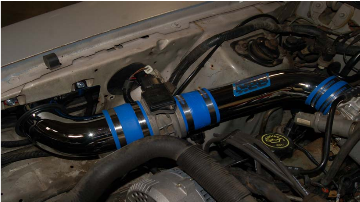
Fig. 8 Install supplied blue connectors and 3" chrome tube. Position tubes for best fit and tighten the clamps.
