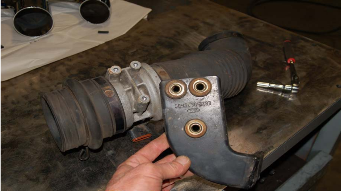
Fig. 3 Remove old Mass Air housing mounting bracket.
