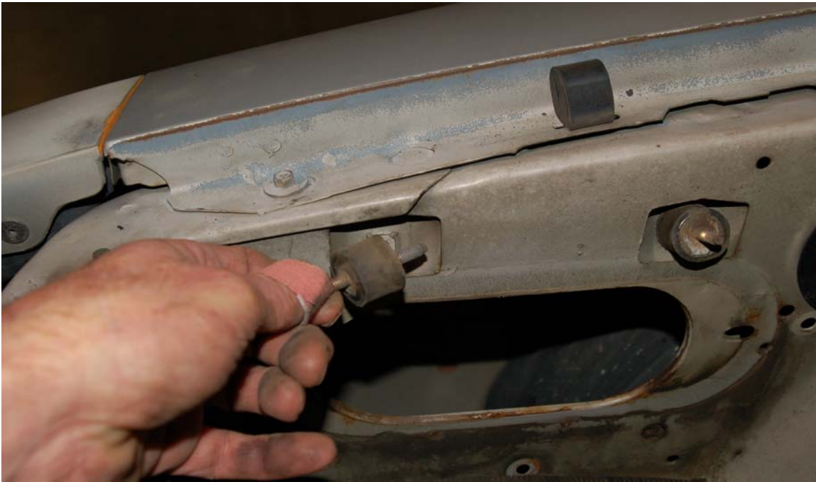
Fig. 2 Remove the rubber bushed studs
