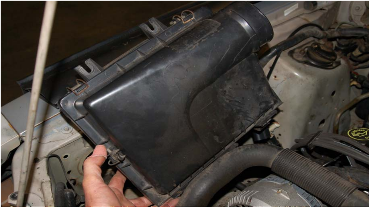
Fig. 1 Removing the stock air box assembly
