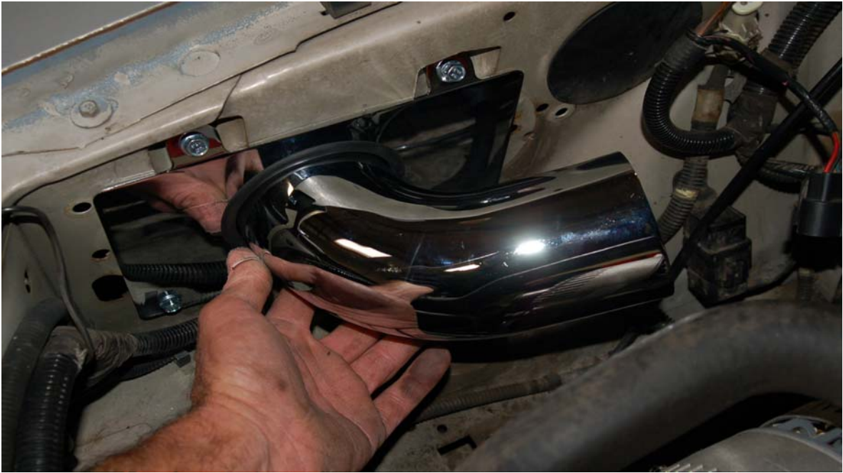
Fig. 7 Lightly oil the rubber O-ring and install the 3 ½" tube.
