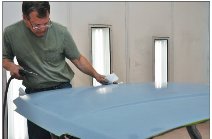
In addition to wiping down surfaces with a tack cloth to catch any dust and other fallout before laying down a final primer coat and paint, Scott notes, the floor in your paint booth should be wet to reduce static electricity and minimize dust particles.
