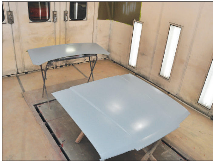
Components, such as the hood and decklid, have been fully prepped and are in the final primer coat before paint. Scott stresses cleanliness, meaning before you lay down primer/sealer wipe down surfaces with a tack cloth and blow off with compressed air.
