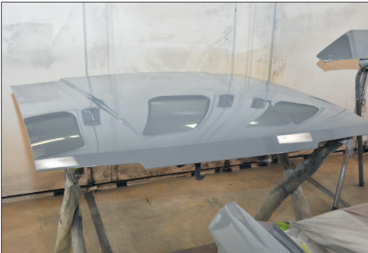
This is what fresh Glasurit primer/sealer looks like after it has been applied. When it cures, it will be a satin finish. This is a two-part primer/sealer when a catalyst is mixed with the paint, and in that case it cures like body filler does.
