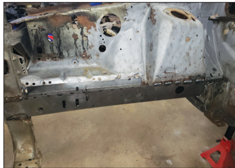
The inside of the frame rail has been replaced and rosette-welded together. A rosette weld, also known as plug-and-fill welding, works wonderfully when you cannot spot-weld these parts together.
