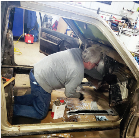
The firewall (also called a dash panel by Ford) and frame rail extensions have been cleaned up in preparation for the Dynacorn floorpan. A good primer-sealer you can weld through has been applied to the contact surfaces.
