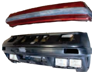
New and used body parts are available for 1979–1993 Mustangs. Here's a rear bumper cover and reproduction fascia for a 1985–1986 Mustang. These need to be prepped and painted off the body. You will also want to use a flex agent in the paint for urethane body parts.
