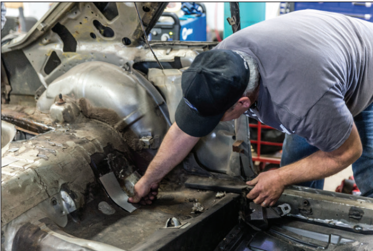
Not all Fox Mustang sheet metal is available, and you may need to hone your fabrication skills. If you have to patch rust holes, make sure all rust is gone; otherwise you're burying an issue that will bite you later. Make sure the patch makes sense and that it will blend nicely.
