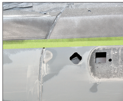
Masking tape is used here to define edges that must be finished in a straight line, because this is one of the first things you see getting into the car.
